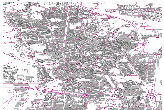
Figure 2: Digital 3D model of a city as input for noise simulation
